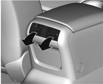
The dashboard and console vents can be adjusted up or down and left or right to allow directional air flow.
