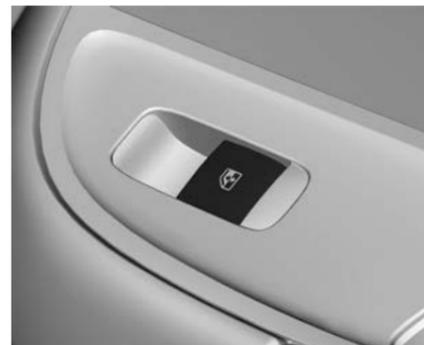
Pushing or pulling lightly to the first detent: window moves down or up as long as switch is operated.
