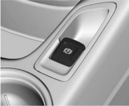
The electric parking brake (EPB) switch is located between the front seats.
