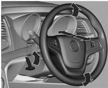
1. Move the lever down to unlock.
