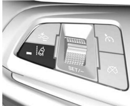
To turn LDW on and off, press the
