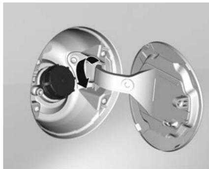
2. Remove the LPG filler dust cap by rotating anticlockwise.
