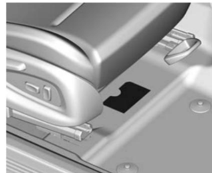
Each vehicle has its own, individual International Standards Organisation Vehicle Identification Number (ISOVIN), which is shown behind the windscreen on the left side and under the right front seat, under a carpet flap.
