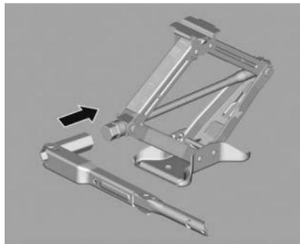
18. Unfold the wheel wrench so it forms a right angle.
