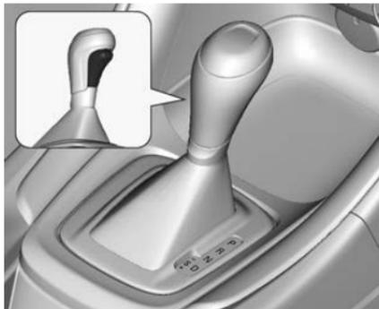
Press the select button on the front of the shift lever to move into any position.
