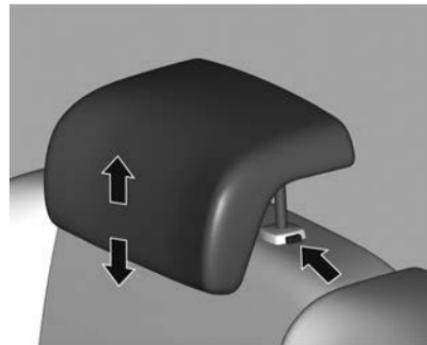
The vehicle may have adjustable rear head restraints, these can be removed.
