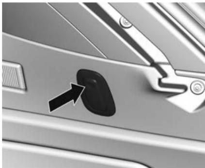
1. To fold the hook out, push in at the top and release it.
