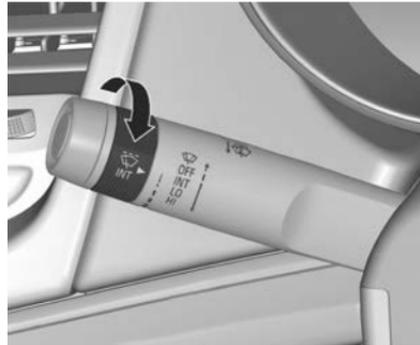
Rotate the collar down for more frequent wipes. Rotate the collar up for less frequent wipes.
