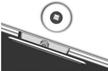
To open the tailgate, access the cargo area from inside the vehicle.
