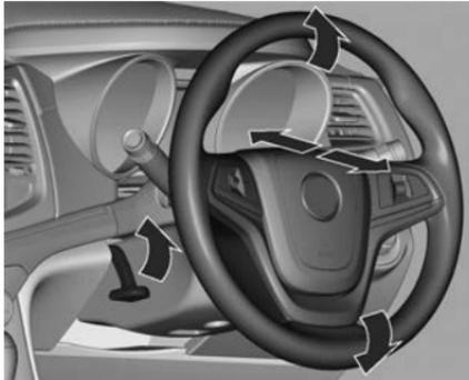
1. To unlock, move the lever down.
