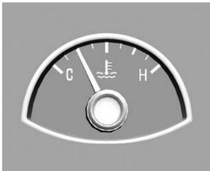
This gauge shows the engine coolant temperature when the ignition is on.
