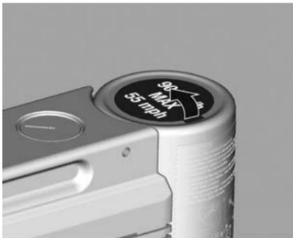
19. After inflating the tyre, remove the maximum speed label and place it in a visible location on the instrument panel.
