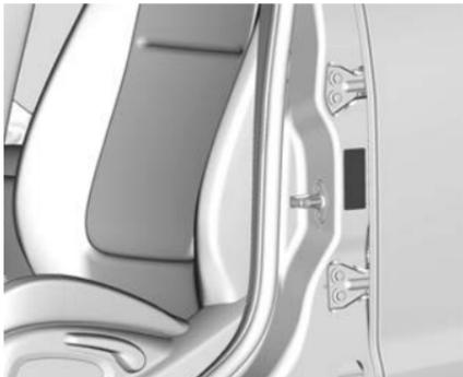
This label shows the vehicle make, model series, date of manufacture, Vehicle Identification Number (VIN), approved seating capacity and approval number.
