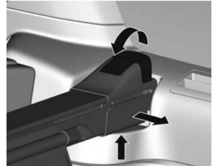
1. On the driver side, lift the lock lever upward.
