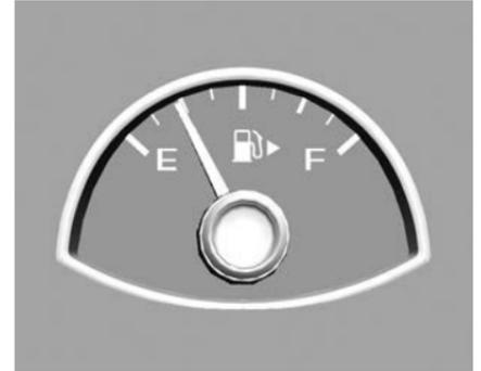
When the ignition is on, the fuel gauge shows how much fuel is left in the fuel tank. When the indicator nears empty, a message in the Driver Information Centre (DIC) displays. See *Fuel System Messages* on page 5-29. An arrow on the fuel gauge indicates the side of the vehicle the fuel door is on.
