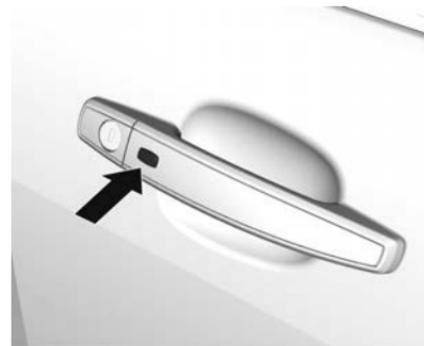
Pressing the lock/unlock button will cause all doors to lock if any of the following occur:
