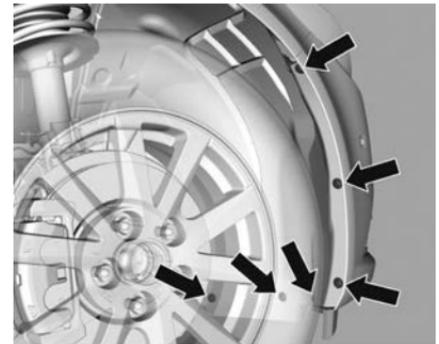
2. Using the torx tool from the toolkit, see *Tools on page 10-38*, remove the six screws at the front of the wheel arch liner.
