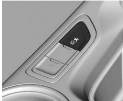
To disable both traction control and ESC, press and hold the button for 5 seconds.
