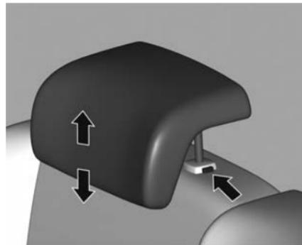
The vehicle may have adjustable rear head restraints, these can be removed. See *Child Restraint Systems* on page 3-20.
