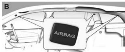
Curtain airbags are stored in the roof on each side of the vehicle.
