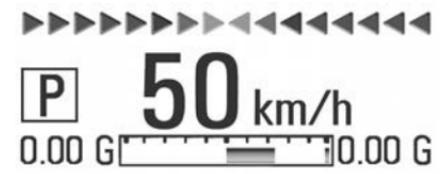
The display at the top of page four shows the gear shift timing. This display will appear with an increase in engine RPM, towards the upper end of the engine RPM range.
