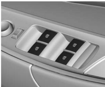
Operate the switch
