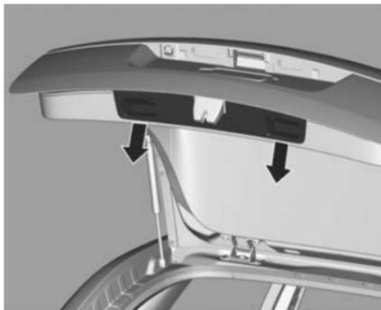
Use the handle to pull down the tailgate until it drops under its own weight. The tailgate closes and latches itself automatically.
