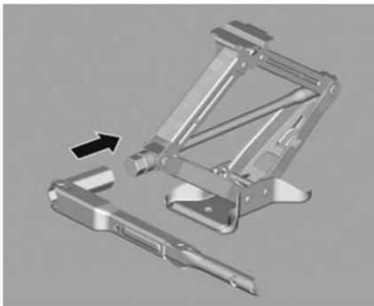
16. Unfold the wheel wrench so it forms a right angle.
