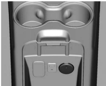
A power socket is located in front of the shift lever and inside the centre console.
