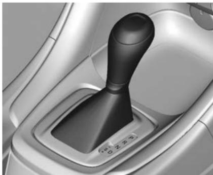
The engine will not start unless the shift lever is in position **P** or **N**.
