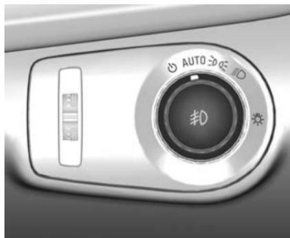
**⏻ (Off):** Turns the headlamps and park lamps off. The switch returns to **AUTO** position. Turn to **⏻** again to re-enable automatic headlamps.
