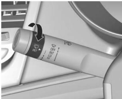
**INT:** The wipers cycle when water is detected on the windscreen.
