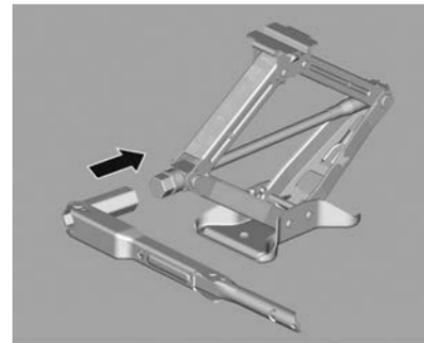
24. Unfold the wheel wrench so it forms a right angle.
