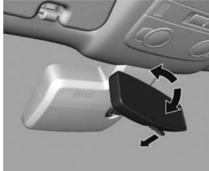
Push the lever on the lower edge of the mirror towards the front of the vehicle, then adjust the position of the mirror.
