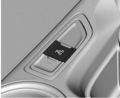
1. With the vehicle in **D** (Drive) or a forward gear, press **P<sup>□</sup>** to initiate APA for a parallel parking space search.
